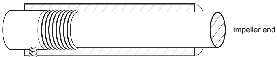
Shaft sleeve threaded to shaft
